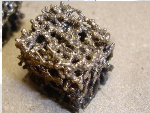
Figure 2. Trabecular implant structure derived from CT data.
