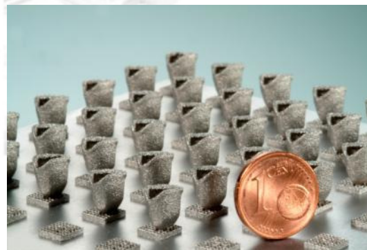
SLM crown production for a fragment of traditional way costs! Over 400 individual units in one shift
